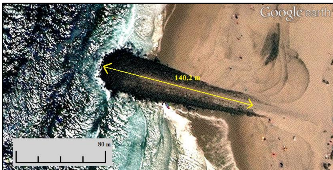
Figure 6.12. Google Earth: distance from the Vagueira North groin tip and the shoreline position at the down drift side of the structure on 18 th of July 2010.
