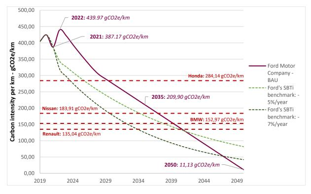
Figure 3.14a. Scenario of evolution for sold vehicles' carbon intensities, compared to SBTi's benchmarks and other company's carbon intensities – BAU
