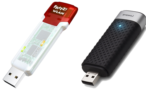
Fig. 2.2: WLAN Fritz! USB card (left side) and Linksys AE3000 USB card (right side).
