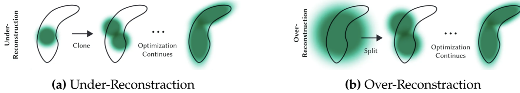
Figure 3.3: Adaptive Gaussian densification scheme. (a) When small-scale geometry (black outline) is insufficiently covered, the respective Gaussians are cloned. (b) If small-scale geometry is represented by one large splat, it is split into two [24].
