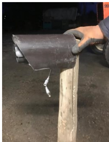
Figure 6. Handmade steel protection used in the experimental trial.
