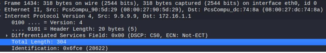
Figure 19 Description of the DNS response packet sent by the open DNS Server
