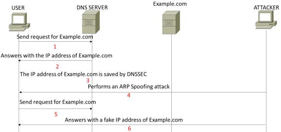
DNSSEC doesn't recognize the IP address of example.com, it blocks the attack and verifies better the source of the message
