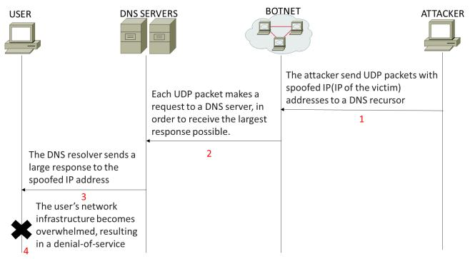
Figure 11 DNS Amplification attack
