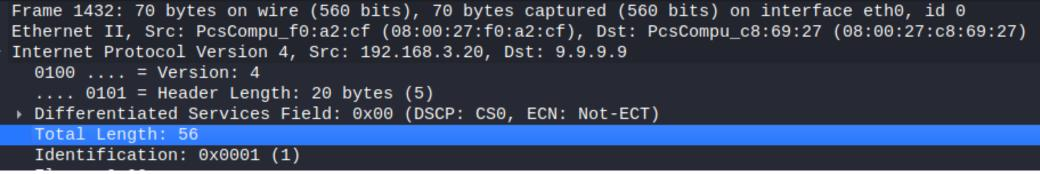
Figure 18 Description of the packet with Wireshark, the total length of the Request packet is 56
