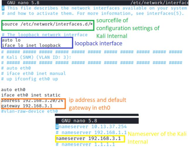
Figure 58 Configuration files network/interface and resolv.conf of Kali Internal
