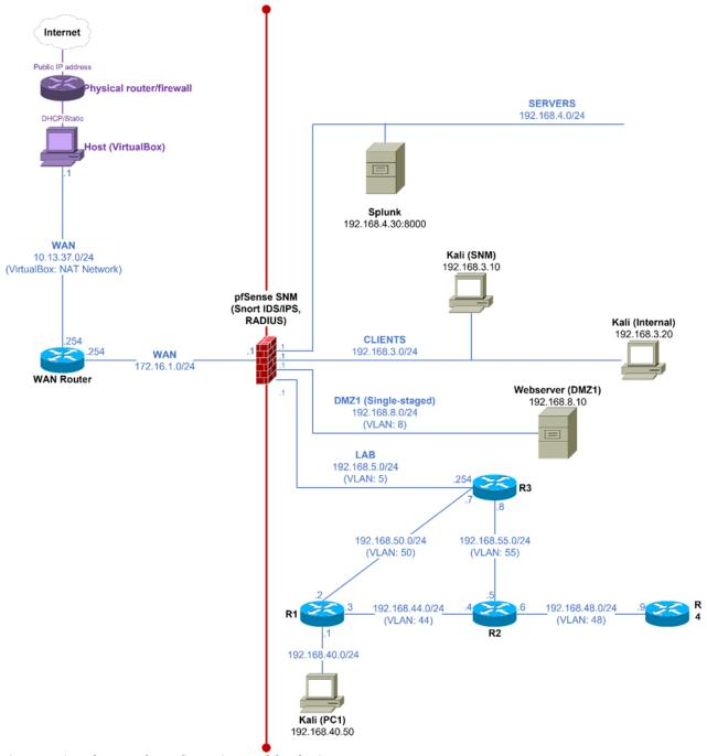
Figure 8 Virtual Network Configuration used for thesis
