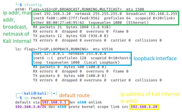
*Figure 57 Results of IP route and ifconfig commands on the kali internal client*
