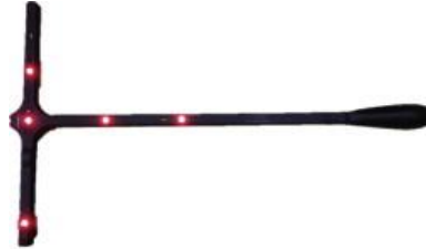
Figure 5. Calibration wand used in the experimental setup. Its active LEDs are automatically tracked by the motion capture software.
