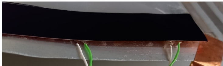
Figure 4-24: Detachment of TiNOX from the TEG.
