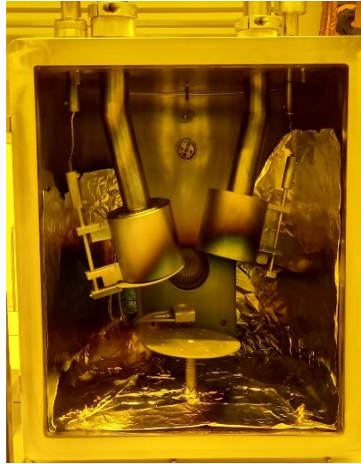
Figure 4-1: IFW magnetron sputtering machine.
