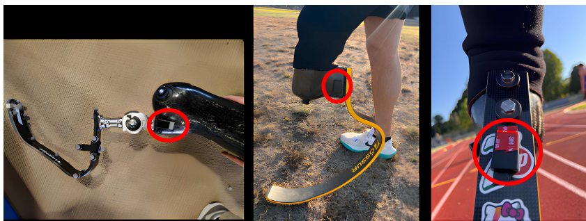
Figure 1.1: Different positioning of the AX6 sensor across subjects: on the left, a Transfemoral (TF) configuration; in the center, a standard Transfemoral (TF) setup; on the right, a custom positioning for a Transtibial (TT) subject.
