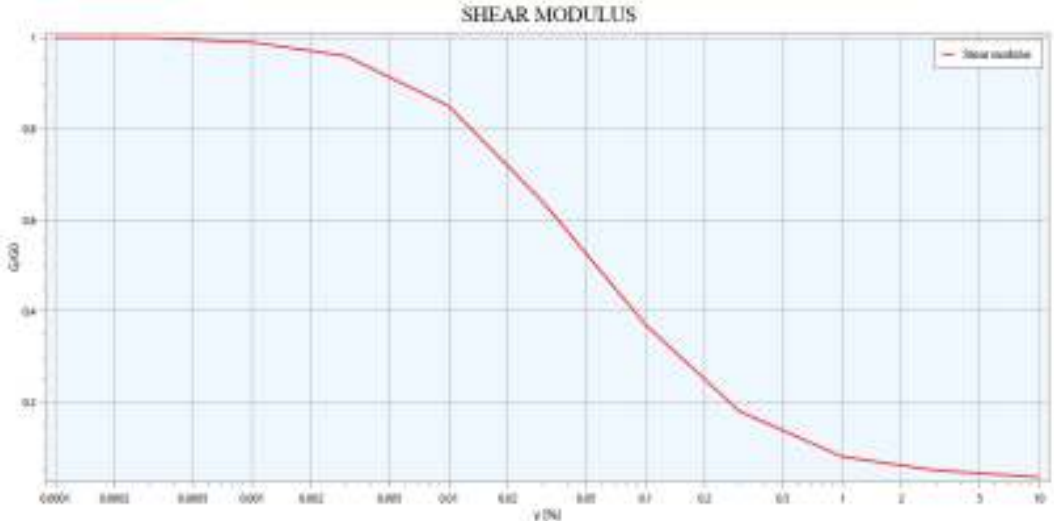
Figure 3.4 - Variation of G with the deformation for a sandy soil
