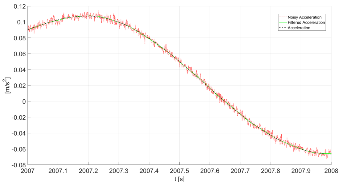
Figure 5.23: Example of comparison between real acceleration, noisy acceleration and a zero-phase filtered version of the latter. The filtered signal provides a good representation of the real acceleration, without presenting any time delay.
