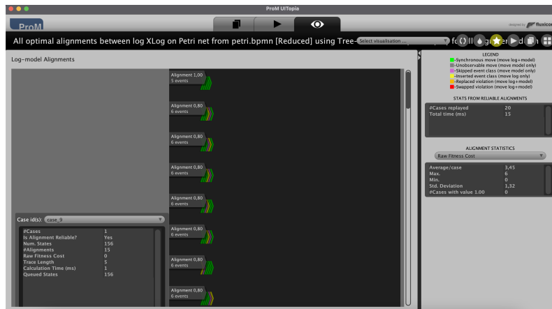
Figure 4.8: Visualization of the result of "Replay a Log on Petri Net for All Optimal Alignments" plug-in. It is computed all the possible alignments of trace case_9 from fitness 1 to fitness equal to 0.8
