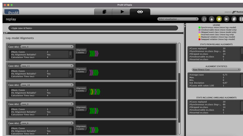
Figure 4.4: Other visualization of the result of our approach implemented in ProM. The plug-in provides the alignments computed using our approach. The green moves are synchronous moves, the purple ones are model moves instead yellow ones are log moves.
