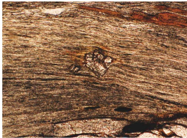
4.11: Staurolite crystals near the edge of a garnet (bottom) under PPL. The base of the photo is 0.68 mm long.
