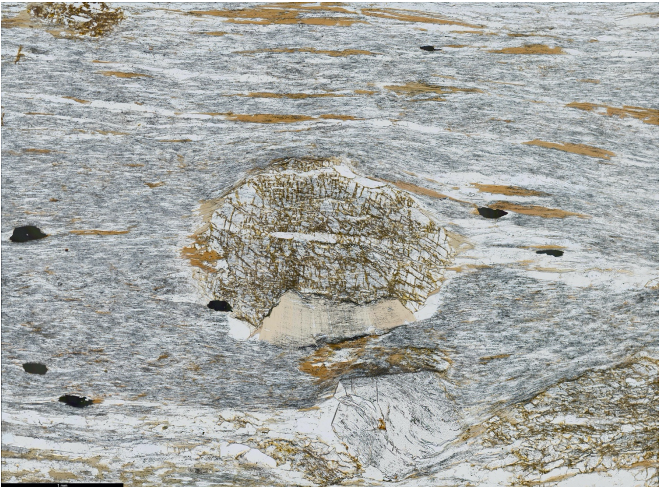
Fig 4.14: carbonate crystals under PPL in sample VIZ07-5P. The black bar is 1 mm long.
