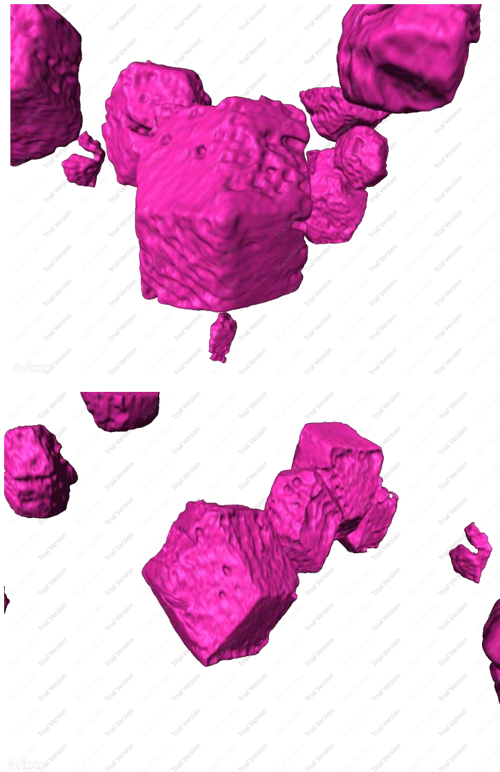
Fig. 4.47: two views of a 3D render of a euhedral rhombododecahedral garnet. The facets are clearly distinguishable, hence the definition of the symmetry.
