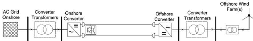
Figure 2.3: Point to point HVDC link
