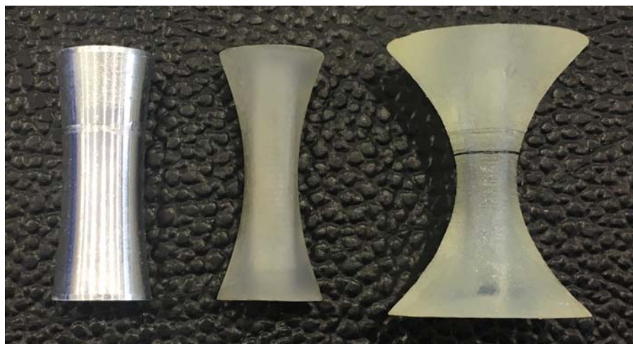
Figure 3.2: DH rollers - from left to right: (i) default Steel roller; (ii) customly printed roller with approx 50% reduced middle section and same tip sections, compared to the default one; (iii) customly printed roller with approx 50% reduced middle section and double tip sections, compared to the default one.
