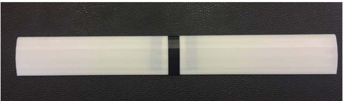
Figure 4.13: Mounted 0.4 m long NACA 0021 blade. The junction between the two 0.2 m parts is reinforced with a 0.06 m internal chunk and sealed for enhanced rigidity.
