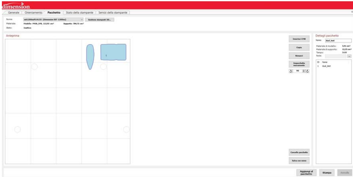
Figure 2.19: Printing package of two 3 cm long NACA 0021 blade chunks. The components are built with a (8; 8; 10) mm Grid Topology Lattice structure and 0.25 mm thick Skin and Lattice Beams. Both horizontal and vertical orientations were considered. A great amount of Support material is required, about twice the Model material volume, because of horizontal configuration and Lattice structure.
