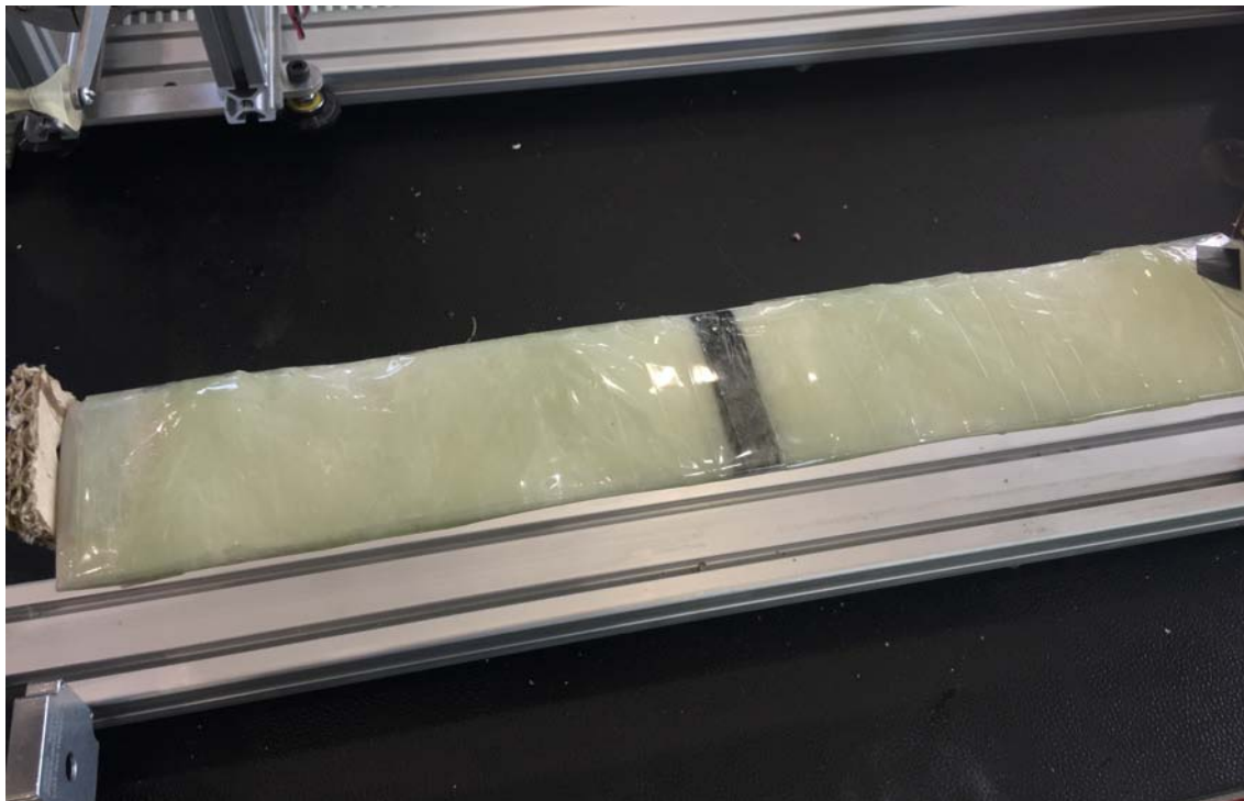
Figure 4.30: GF/epoxy filament wound optimized NACA 0015 VAWT blade demonstrator.
