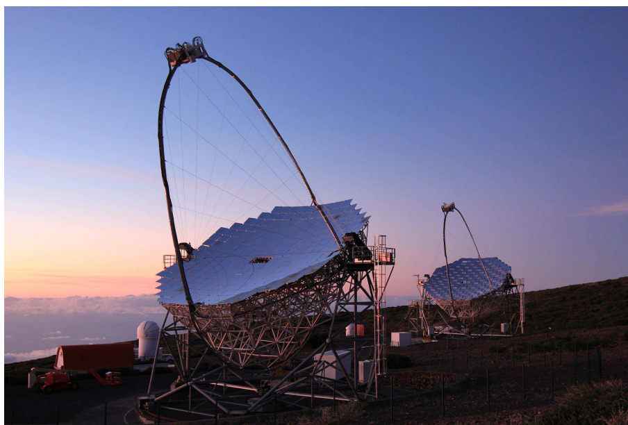
Figure 2.1: MAGIC telescopes, Observatorio Roque de los Muchachos, La Palma, Canary Island, Spain. MAGIC I (left), MAGIC II (right). The project started in 2003 with the construction of MAGIC-I; later in the 2009 a second telescope, MAGIC-II, was added. Since then, the two telescopes worked in stereoscopic mode, making a great improvement in the sensitivity. Credit: Giovanni Ceribella.
