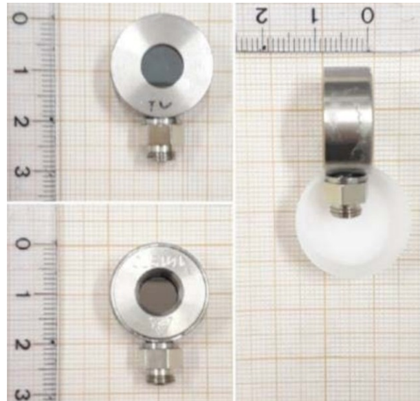
Figure 2: Picture of one of the PIPS diodes used for heavy-ion beam characterization, shown in top, bottom, and side views. The stainless-steel package and the front aperture above the active area are visible. Reproduced from [6].
