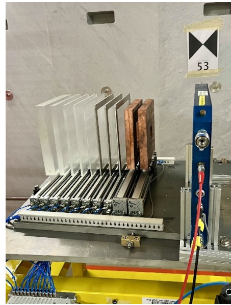
Figure 6: Example of the PMMA degrader system used in the HEARTS@CERN campaign to generate additional effective-energy conditions upstream of the PIPS diode. Reproduced from [6].
