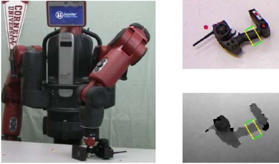
Figure 5.4: A robot grasping an object (left), the object grasp in RGB and depth images (right).
