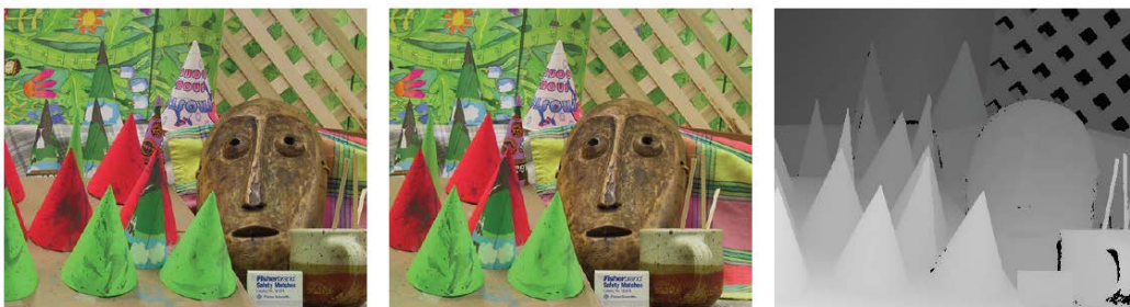
Figure 2.2: Image captured by the left camera (left), image captured by the right camera (center) and the computed disparity map (right).
