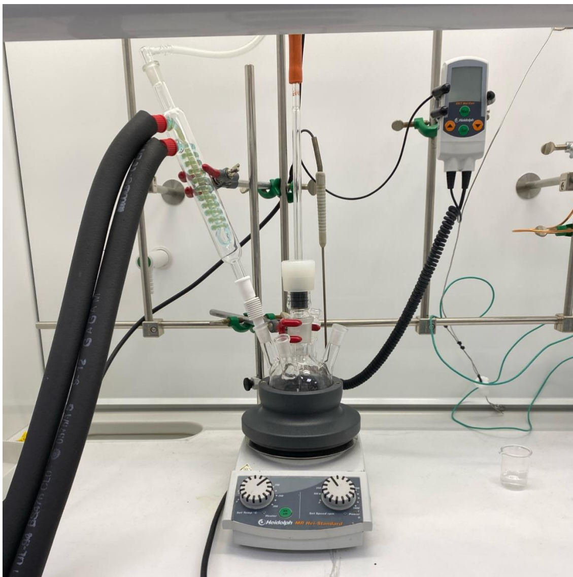
Figure 59. Experimental apparatus used for the reduction of the first batch of bifunctional catalyst, consisting in a glass reactor, a cryostat, a mechanical stirrer and a thermometer.
