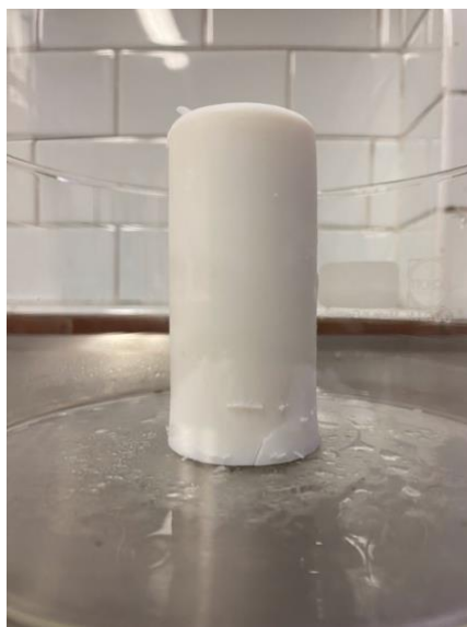
Figure 18. Monolith of polydivinylbenzene after the polymerization.
