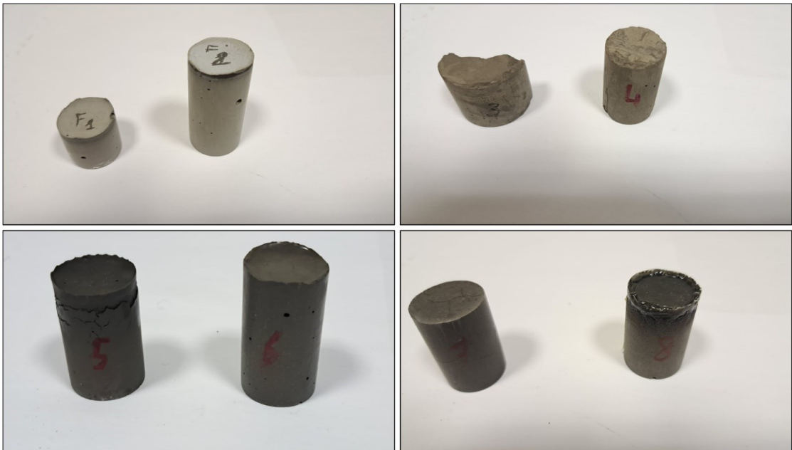
Figure 2.1. Hardened samples of simulant regolith with a diameter of 2 cm.
