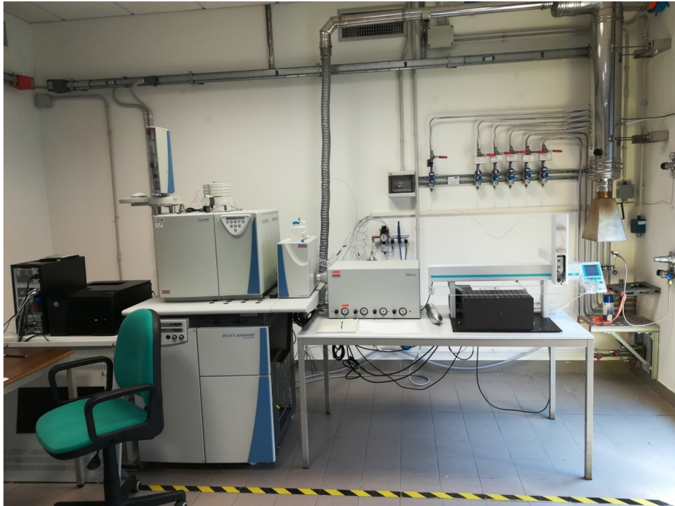
Fig. 12: Mass spectrometer Delta V Advantage (Thermo Scientific) connected with a Gasbench II device. Department of Geosciences, University of Padua.
