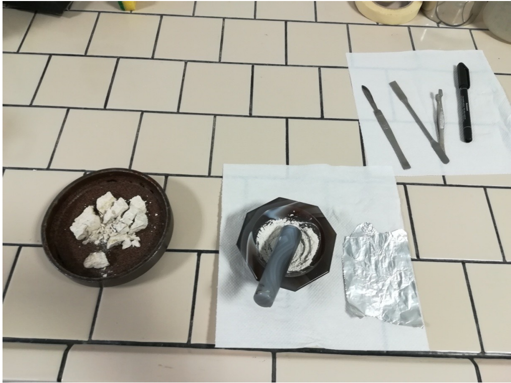
Fig. 11: For bulk analysis the chips obtained with a crusher have been ground in an agate mortar.
