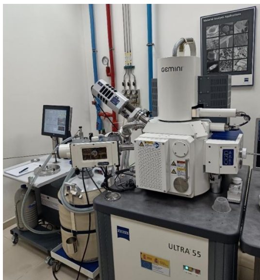
Figure 9. Cryo-SEM microscopy composed by the Zeiss Ultra 55 body and the Quorum PP3010 sublimation chamber.
