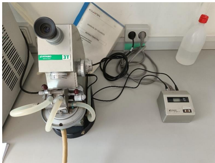
Figure 8. Atago 3T with Polyscience temperature controller for the determination of TSS
