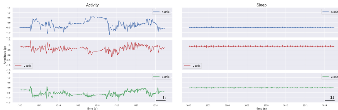
Figure 3.4: Accelerometer signals during activity and sleep. Each row indicates a different accelerometer axis. The two columns represent an example of activity epoch and one of sleep.
