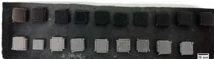
(b) After pyrolysis (incomplete pyrolysis).
