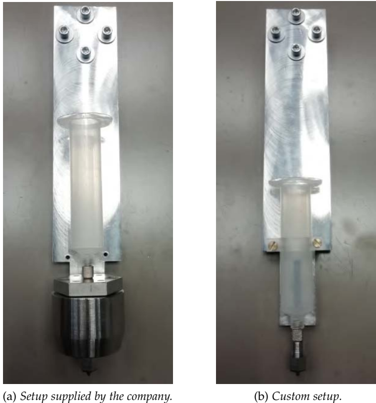
Figure 2.16: Different adapter arm setups for single paste robocasting.
