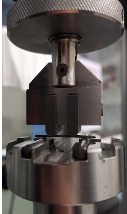
Figure 2.13: Instron 4204 UTM setup for bending test (support span=20 mm, load span=10 mm).
