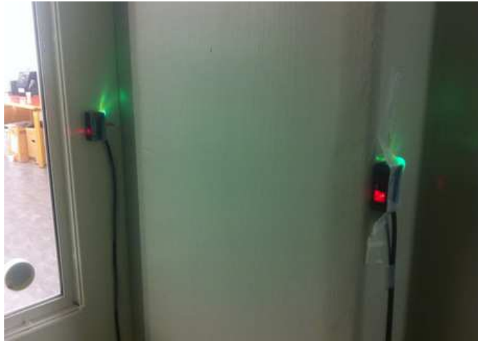
Figure 4.13: Photoelectric device used in the people counter system.
