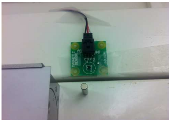
Figure 4.14: Magnetic device used in the people counter system.
