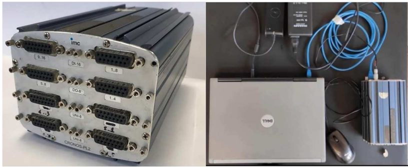
Figure 6.7: On the left there is an image of the strain gauge control unit IMC. On the right, there is an image of the system for the acquisition (personal compute, strain gauge control unit and relative cables).
