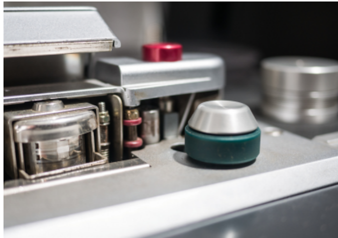
Figure 2.3: Tape scrolling mechanism of the Studer A810.
