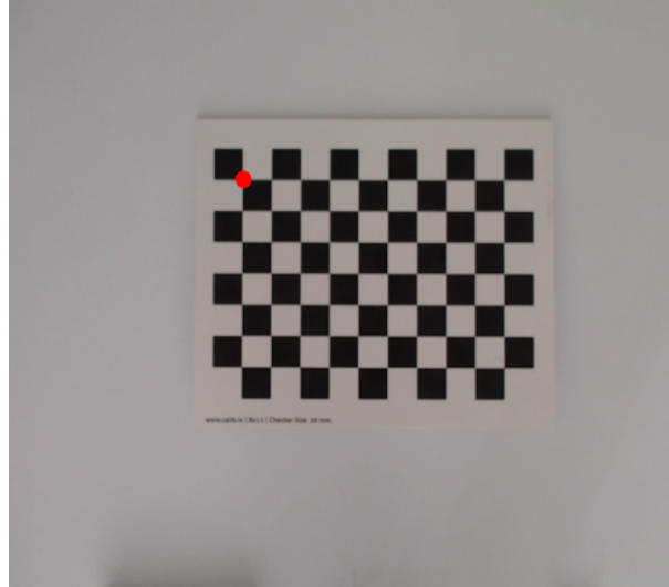
Figure 3.7: Result of the camera matrix equation validation
