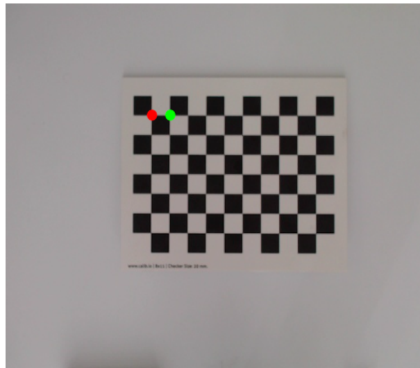
Figure 3.8: Points for the inverse camera matrix equation validation
