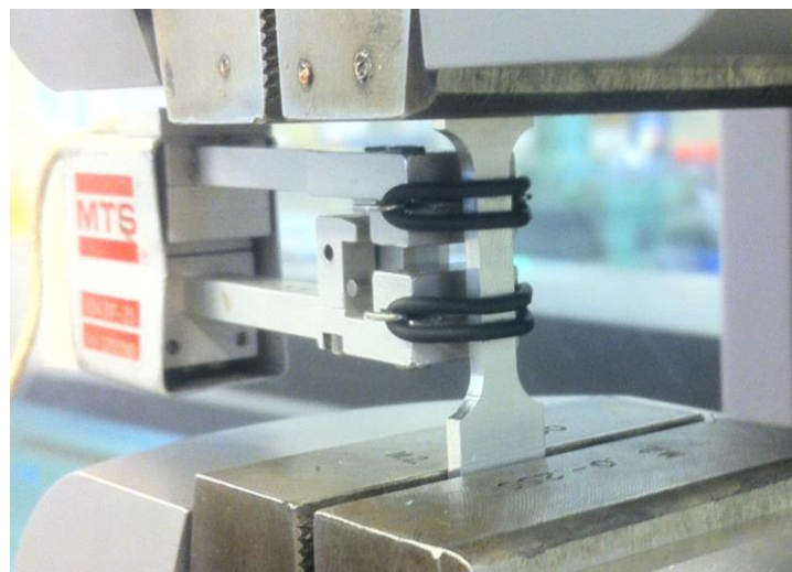
Fig.66 Testing of the BM with the extensometer
