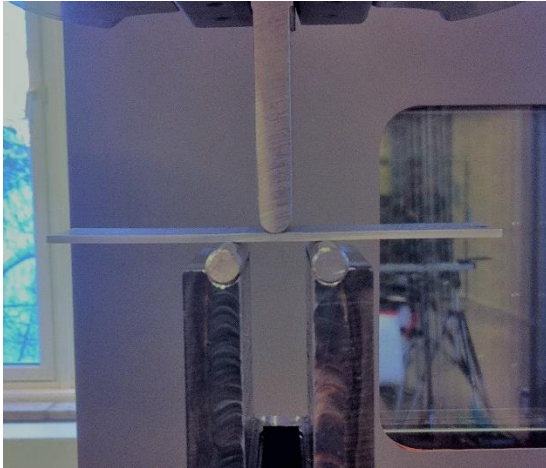
Fig.46 Before the bending test
