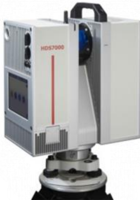
Figure 3.12. The laser scanner Leica HDS 7000 used for the scanning of the lava tube of La Corona.
