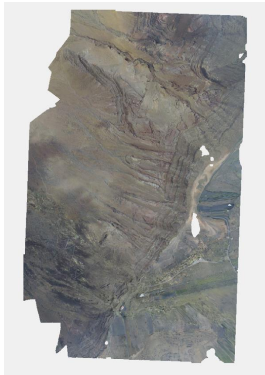
Figure 3.10. Orthomosaic obtained with Photoscan of the area next to the Camino de Los Gracioseros with the resolution of 0,90 m.
