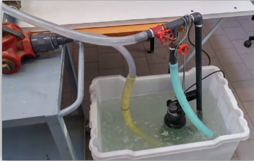
Figure 2.5: water tank with the pump
