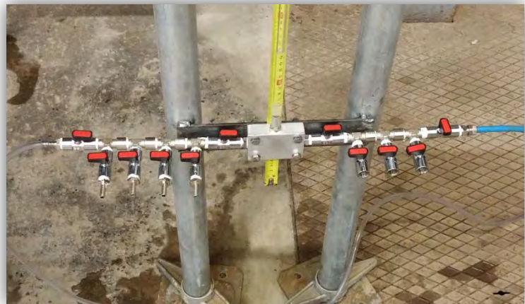
Figure 3.5: attachment of the pressure sensors
