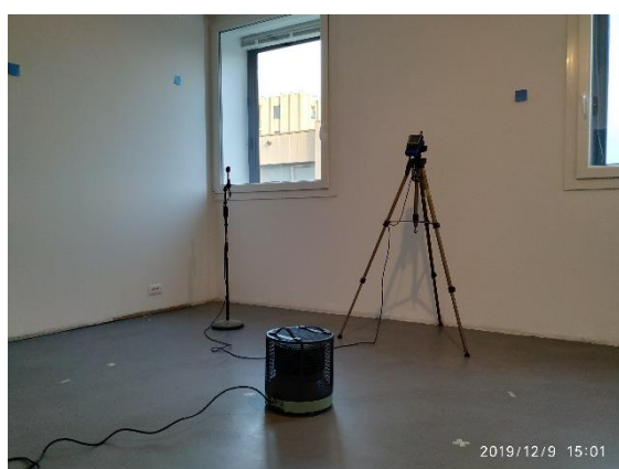
d) Close up of Reference Sound Source for sound power level determination.
