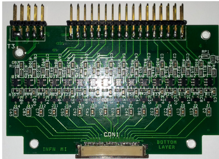
Figure 4.10: Low-noise charge sensitive preamplifier for the DSSSD detector.
