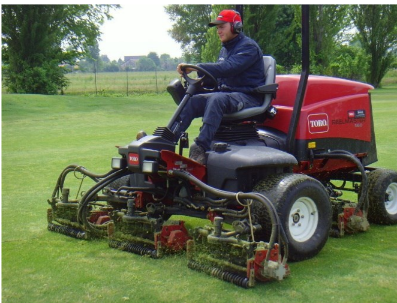
Figura 28. Quintupla Montecchia (TORO 5510-D 5-Gang Reel Fairway Mower).
