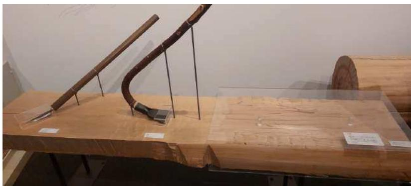
Figure 97 Tools displayed in the position of use. The wood shows the marks the instruments create in its superficies. As these are instruments with sharp blades, the cutting edges were protected with acrylic cases. Photo: author.
