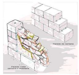
Figure 80 Example of the use of the pedra e cal masonry and the cantaria. Source: Colin [2010]. 297
