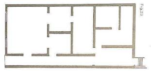
Figure 35 Plan of house in Ouro Preto that shows the corridor connecting the entrance and the back door. Source: Vasconcellos [2010].<sup>213</sup>
