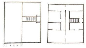
Figure 38 Plan of the two floors of a *sobrado* of Ouro Preto. Source: Vasconcellos, 2010.<sup>217</sup> In the 19<sup>th</sup> century, the houses maintained mostly the same typologies of the 18th
