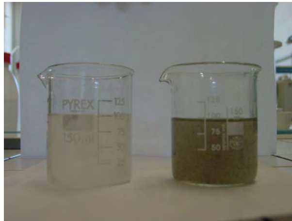
Figure 3.22: Feed in the reactor at the beginning of the short-term test and the solution at the end.
