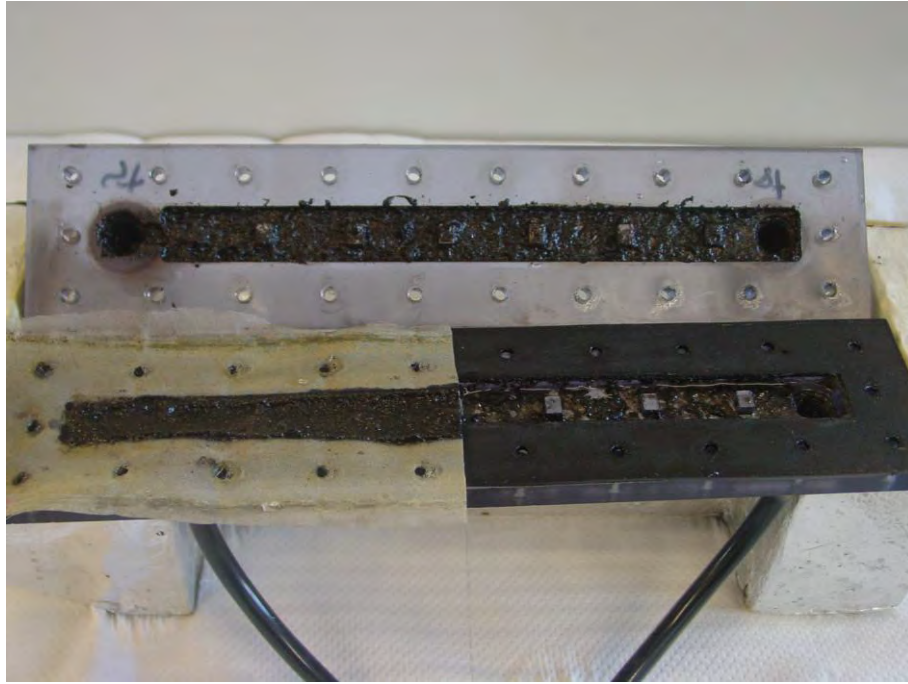
Figure 3.24: Membran esupport after the shutdown. The mesh and the lower side of the device can be seen properly.
