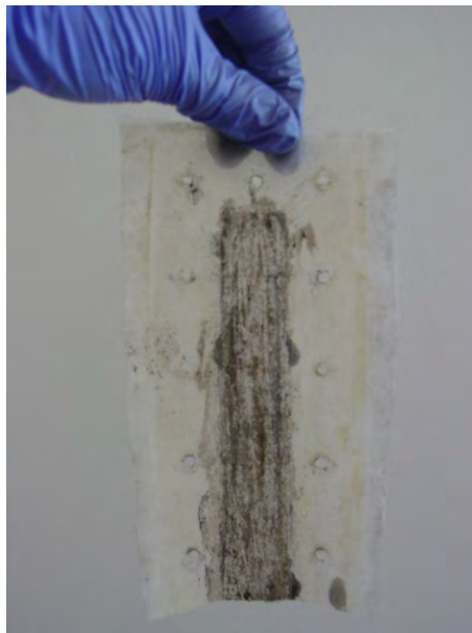
Figure 3.5: Image of the support mesh after cake layer scouring. The biofilm layer developed on the mesh can be noticed.
