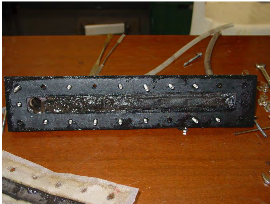
Figure 3.1: the upper part of the membrane support on day 17. On the left it is possible to notice the sludge clogging the device.
