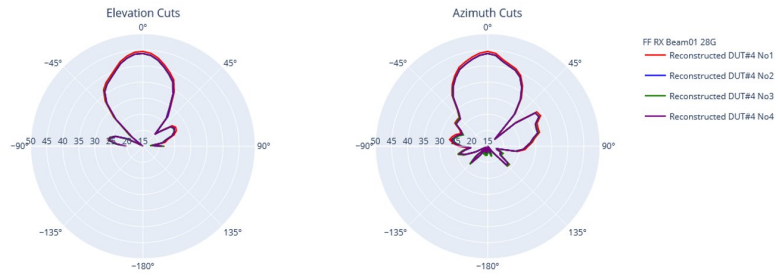
Figure 2.17: Beam 1 at 28 GHz - repeatability of the measurements
