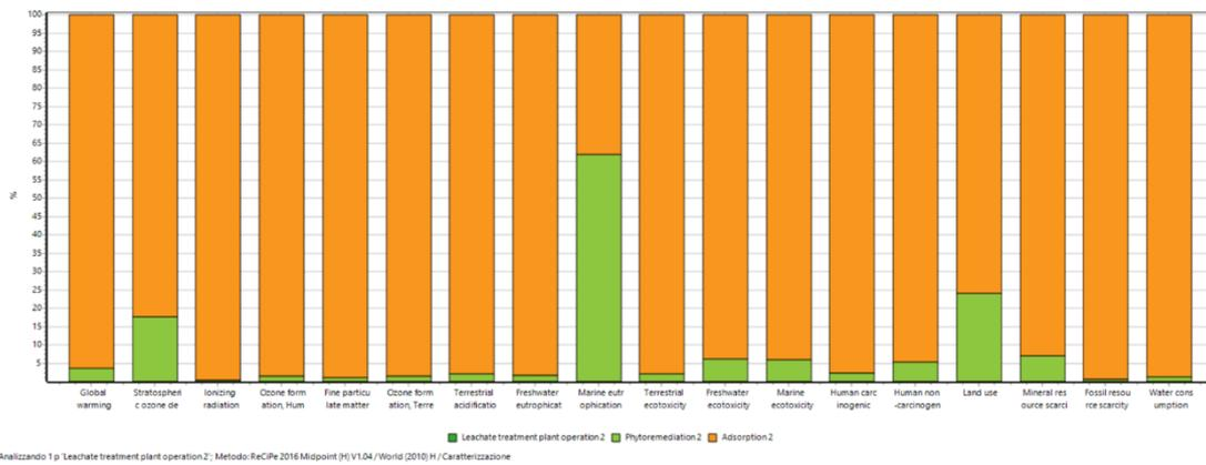
Figure 62. Graphical representation of characterization results through ReCiPe 2016 method for leachate treatment plant operation during the aftercare (personal elaboration from SimaPro software).
