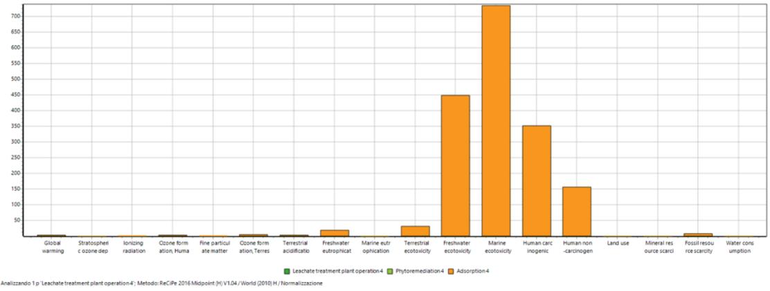
Figure 78. Graphical representation of normalization results through ReCiPe 2016 method for the leachate treatment plant operation during landfill conversion (personal elaboration from SimaPro software).
