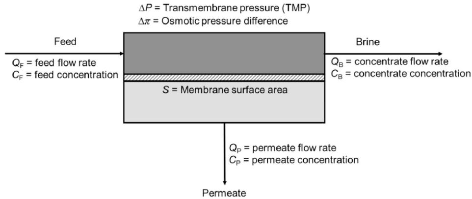
Figure 6. Schematic of a continuous RO system (Qasim et al., 2019). In the image the concentrate is called brine.
