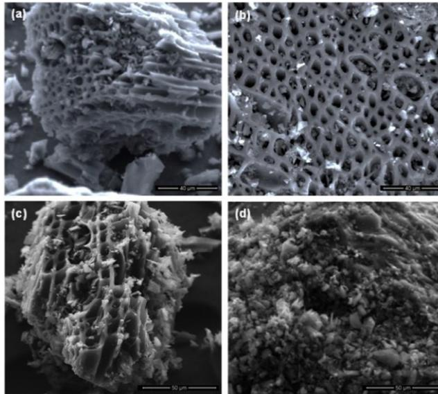
Figure 15. Scanning electron microscope images of conocarpus pruning waste activated carbon (a) activated with KOH, (b) activated with ZnCl<sub>2</sub>, (c) non-activated, (d) commercial activated carbon (Reshadi et al., 2020).
