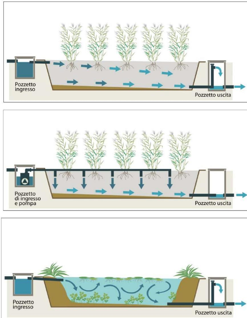
Figure 12. Types of flows in phytoremediation basins: horizontal flow, vertical flow, free water (ISPRA, Manuali e Linee Guida 81/2012).
