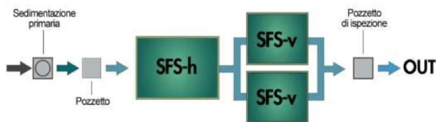
Figure 13. Diagram of a hybrid HF + VF phytopurification plant in series (ISPRA, Manuali e linee guida 81/2012).
