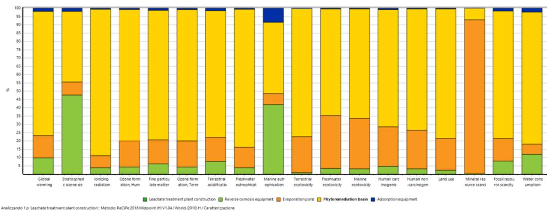
Figure 44. Graphical representation of characterization results through ReCiPe 2016 method for the leachate treatment plant construction (personal elaboration from SimaPro software).
