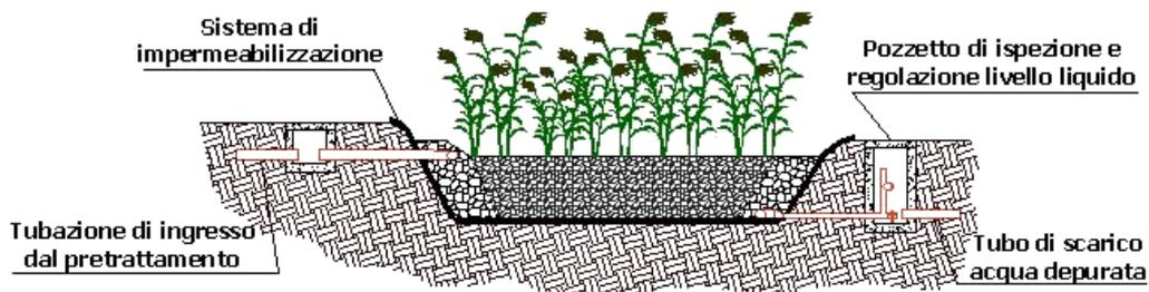
Figure 39. Longitudinal section of a phytoremediation basin. Detail of the impermeabilization and irrigation system; distribution of the substrate (gravel of coarse-medium size)(Source: unknown).
