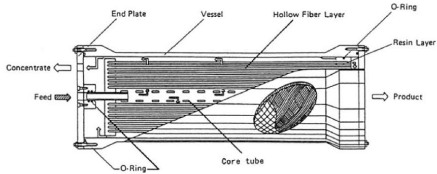
Figure 7. Hollow fiber RO membrane module (Qasim et al., 2019).
