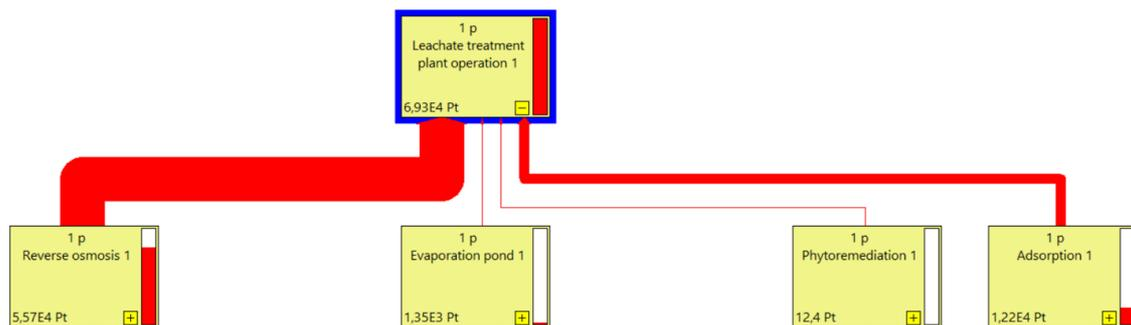
Figure 52. Leachate treatment plant operation during filling input/output analysis (personal elaboration from SimaPro software).
