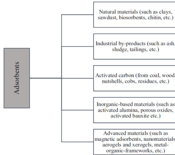
Figure 14. A simple classification of adsorbents (Reshadi et al., 2020).
