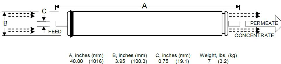
Figure 30. Detail of membrane dimensions (Hydronautics, Nitto Group Company).
