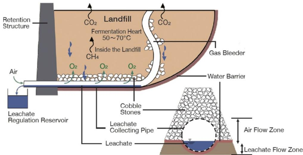
Figure 2. Simplified scheme of a semi aerobic landfill (JICA, 2007).
