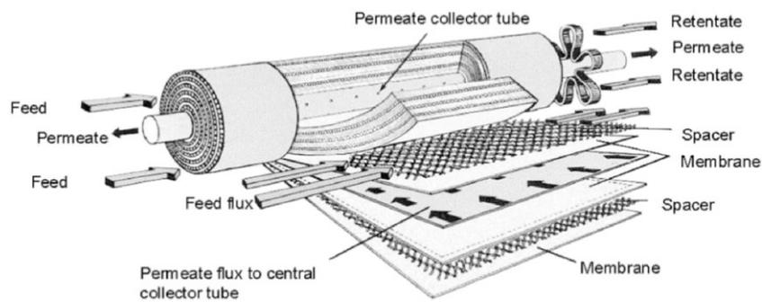
Figure 8. Spiral wound RO membrane module (Qasim et al., 2019).
