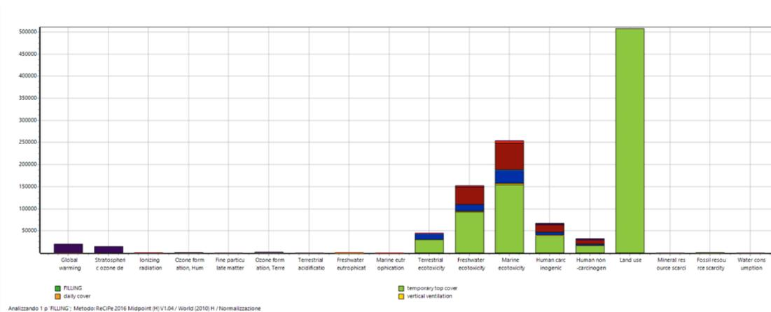
Figure 60. Graphical representation of normalisation results through ReCiPe 2016 method for the landfill filling (personal elaboration from SimaPro software).
