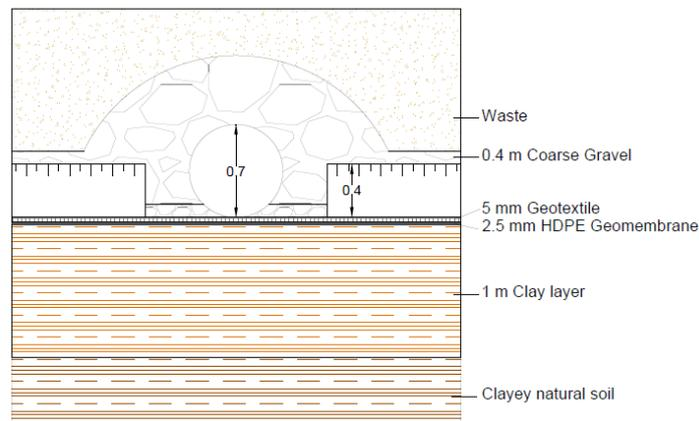
Figure 19. Primary pipes details (Lazzarin, 2015/2016).
