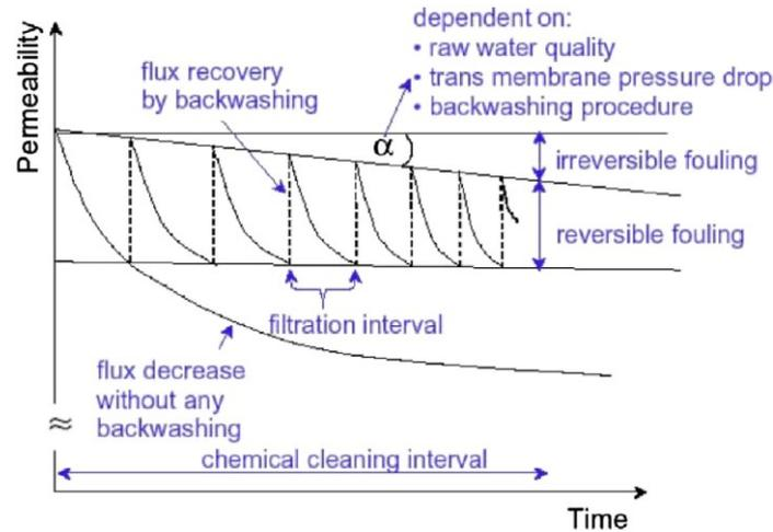
Figure 9. Principle of flux decrease without backwashing and cleaning. Flux recovery by backwashing and resulting elimination of reversible fouling and remaining irreversible fouling (Cossu and Stegmann, 2018).
