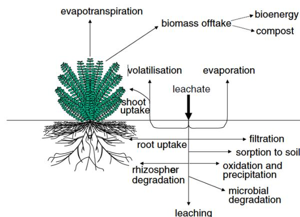
Figure 11. Schematic representation of the soil-plant bioreactor for the plant-soil based treatment of landfill leachate (Jones et al., 2005).
