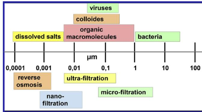
Figure 4. Dimension range of different water compounds (mm) (upper part) and permeation range of different membrane processes (Cossu and Stegmann, 2018).
