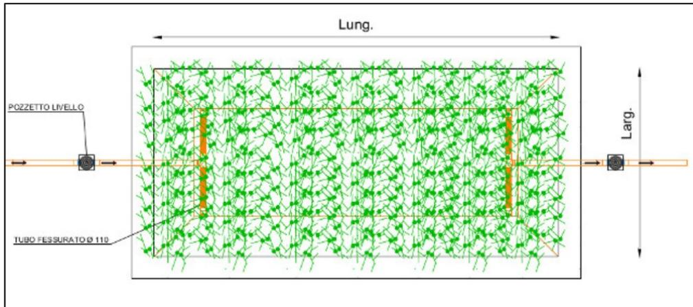
Figure 38. Planimetry of a rectangular phytodepuration basin. Detail of the configuration of the irrigation system. The level well at the outlet collects the leachate to be treated in the secondary basin connected in series at the lower level (Source: unknown).
