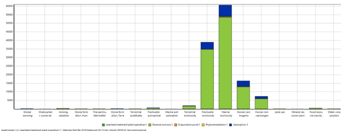
Figure 58. Graphical representation of normalisation results through ReCiPe 2016 method for leachate treatment plant operation during landfill filling (personal elaboration from SimaPro software).
