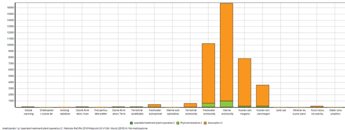
Figure 65. Graphical representation of normalisation results through ReCiPe 2016 method for leachate treatment plant operation during landfill aftercare (personal elaboration from SimaPro software).
