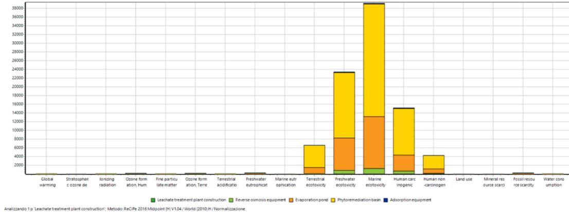
Figure 49. Graphical representation of normalization results through ReCiPe 2016 method for the leachate treatment plant construction (personal elaboration from SimaPro software).
