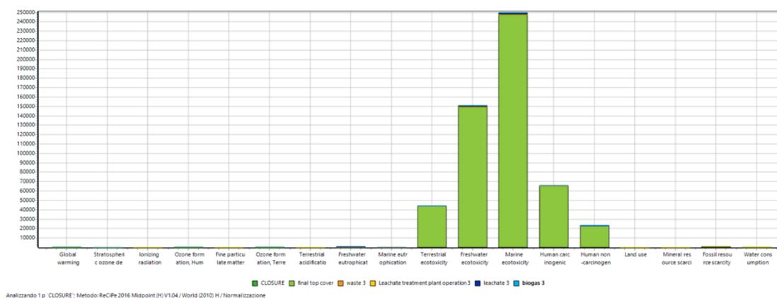
Figure 73. Graphical representation of normalisation results through ReCiPe 2016 method for the landfill closure (personal elaboration from SimaPro software).
