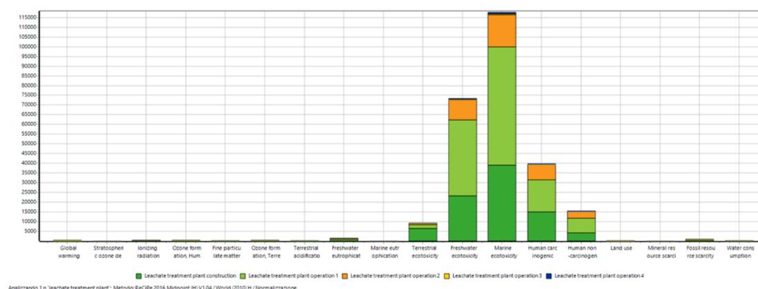
Figure 42. Graphical representation of normalisation results through ReCiPe 2016 method for the entire leachate treatment plant life (personal elaboration from SimaPro software).
