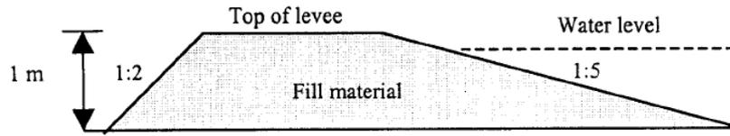
Figure 35. Generalised embankment dimensions (Ahmed et al., 2000).
