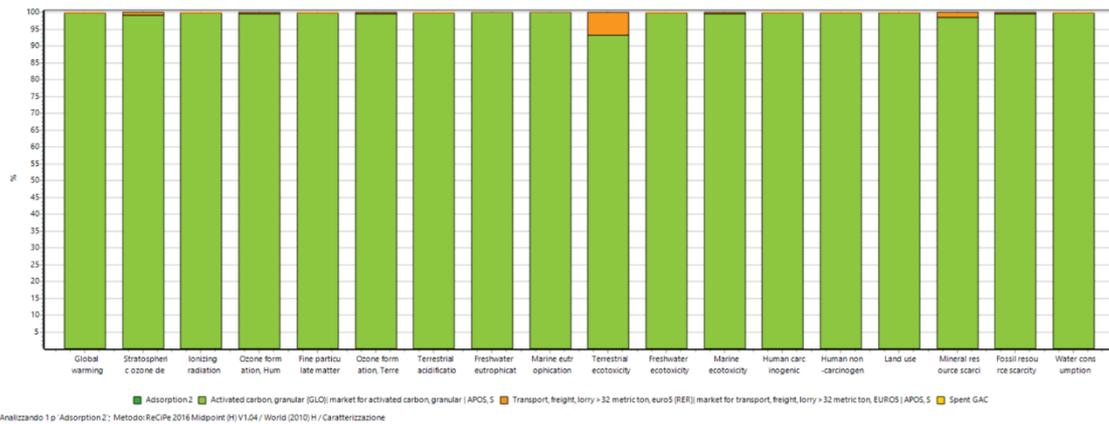
Figure 64. Graphical representation of characterization results through ReCiPe 2016 method for adsorption operation during the aftercare (personal elaboration from SimaPro software).
