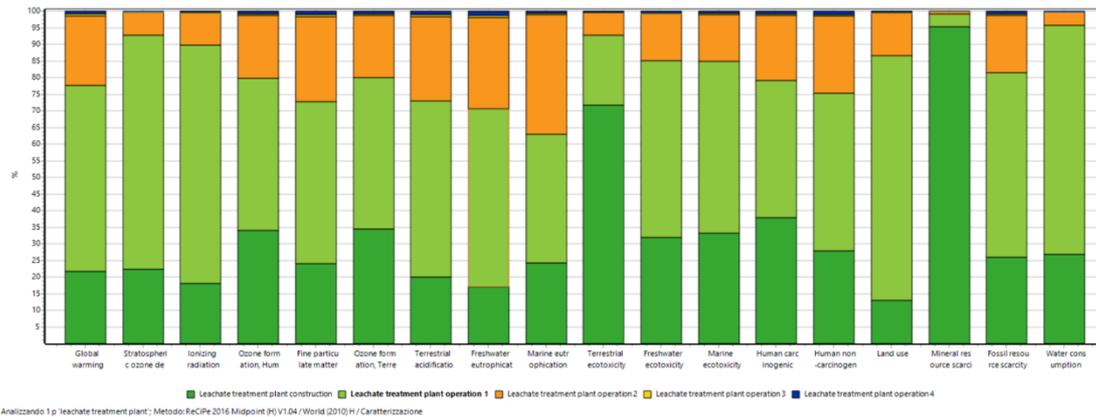
Figure 41. Graphical representation of characterization results through ReCiPe 2016 method for the entire leachate treatment plant life (personal elaboration from SimaPro software).
