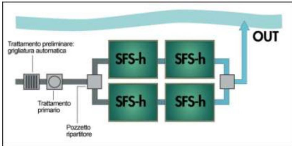
Figure 37. Scheme of an HF constructed wetland plant for urban wastewater (Manuali e Linee Guida 81/2012, ISPRA). In this leachate treatment project, the scheme remains the same as that shown in the figure, while preliminary and primary treatment are to be excluded.
