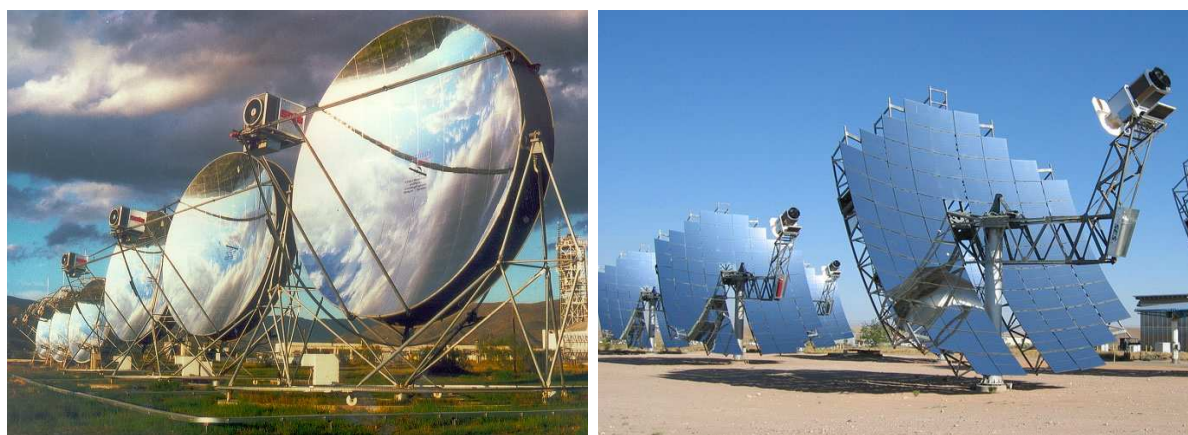
Figure 1.5: Two types of Dish/Engine Systems: Compact Mirror Dishes (on the left) and Multiple Mirror Dishes (on the right). Each of this solar concentrators has a fixed-focus faceted dish with a concentration of up to 250 suns.
