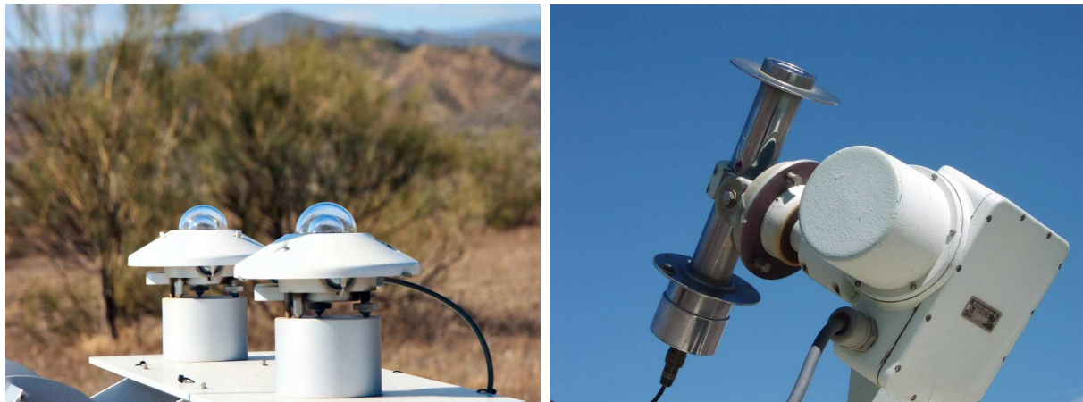
Figure 2.5: Solar devices to measure the two principal components of solar irradiance: Pyranometer, used to obtain the value of global irradiance (on the left); Pyrhelioscope, used to obtain the value of direct irradiance (on the right).
