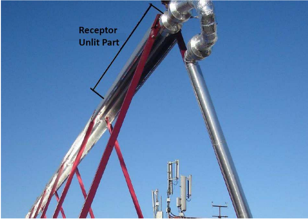
Figure 4.24: Example of receptor unlit part on the east extreme before solar noon.
