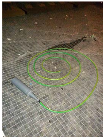
(c) Short narrow tube (length 8.8 m, inner diameter 1.2 cm).
