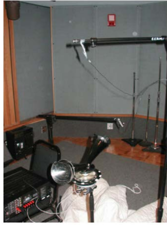
Figure 2.7: Leslie rotating horn.
