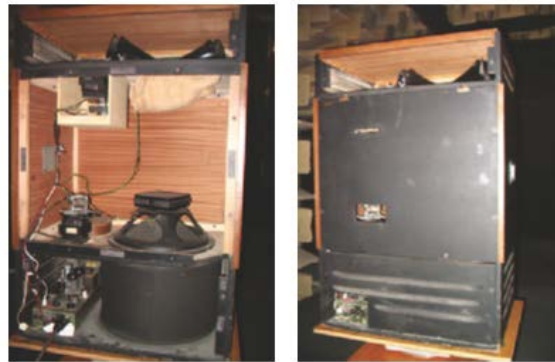
Figure 2.10: The Leslie cabinet used for the measurements: (left) open and (right) closed.
