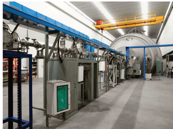
Figure 1.6: On the left, a picture of the Tandem tank, in which can be seen the beam tube and the voltage terminal; on the right, a picture of the final stretch of the accelerator, where the beam is injected in the switching magnets. Pictures taken from [8].
