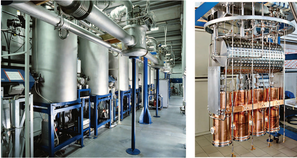
Figure 1.7: On the left, a picture of ALPI and the cryostats; on the right, the interior of a cryostat. Pictures taken from [8].
