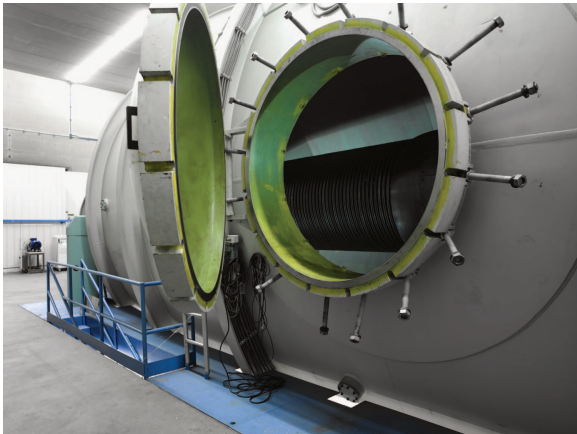
Figure 1.6: On the left, a picture of the Tandem tank, in which can be seen the beam tube and the voltage terminal; on the right, a picture of the final stretch of the accelerator, where the beam is injected in the switching magnets. Pictures taken from [8].
