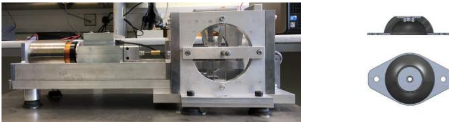
Figure 2.6: The Manipulator (on the left) and the Geometric Representation of the Anti-Vibrational Feet (on the right) [7].
