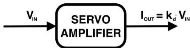
Figure 2.12: Amplifier Method of Operation.
