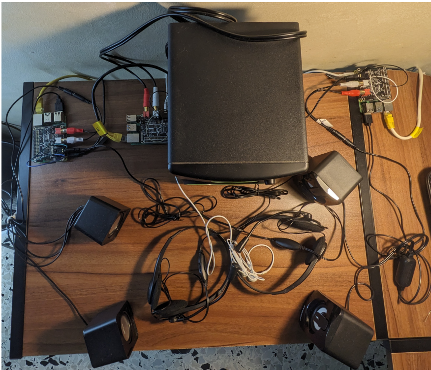
Figure 4.3: Setup using SuM modems, with each modem connected to a set of audio speakers for output, a headset for input and to a switch via Ethernet.
