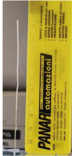
Figure 4.43. Robotic Arm (left). Figure 4.44. Vertical filament (10 cm, 0.4 mm/min), (right).
