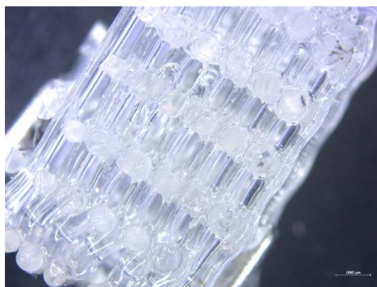
Figure 4.29. Internal section of 6H44-2PETTA scaffold.
