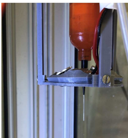
Figure 4.5. Formation of the continuous filament of the ink composition 6H44-2PETTA-2%PI.
