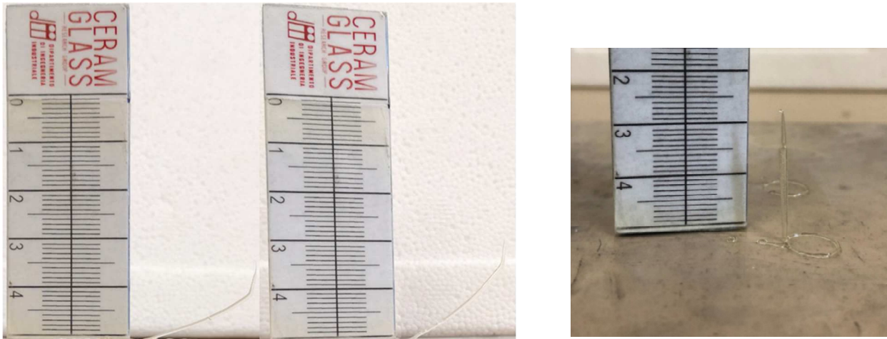
Figure 4.6. Vertical and inclined structures. Filaments inclined by 60°, on the left TEGO on the right PETTA (left). In the image on the right vertical filament of PETTA.
