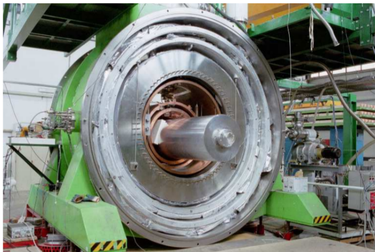
Figure 1.3: The NAUTILUS cryogenic resonant detector (open), installed at the "Laboratori Nazionali di Frascati" (INFN) in the years 1994-2016 operating at 2 K. [1].
