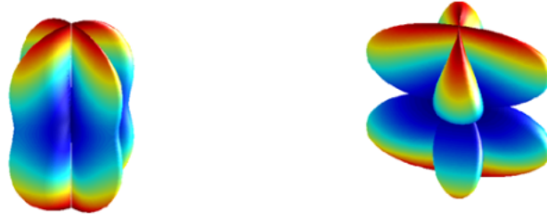
Figure 1.7: The antenna pattern for an interferometer decomposed into its sensitivity in the + polarization (left) and the \times polarization (right) [5].
