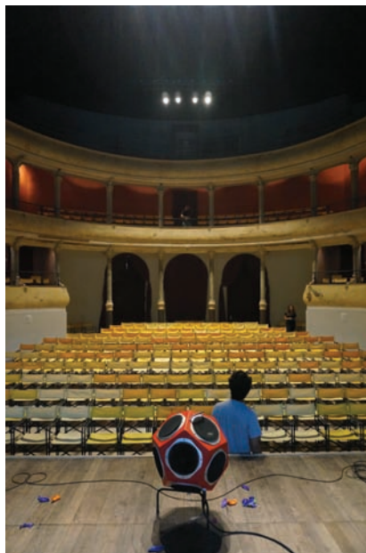
(c) Omnidirectional dodecahedron.
