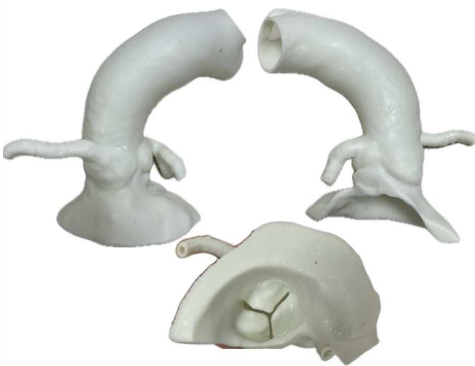
Figure 51 | 3D model of aortic valve in Loctite 3D IND475™ with a biological valve.
