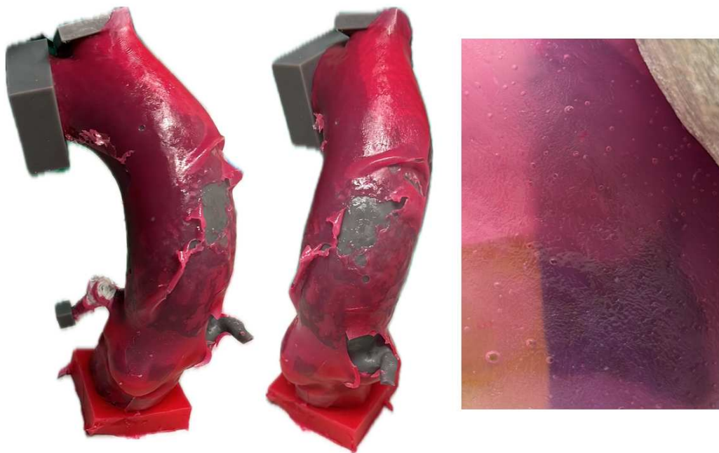
Figure 56 | Final result with the presence of air bubbles inside the silicone highlighted.
