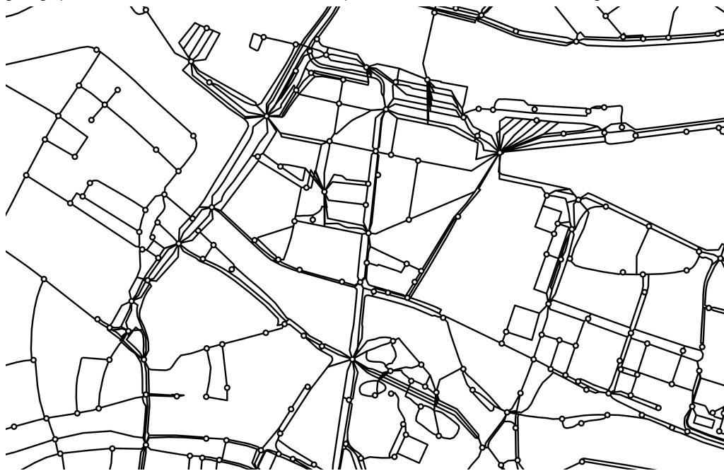
(b) Simplified graph. The administrative area of the Padua city contains 7953 nodes and 14696 edges.
