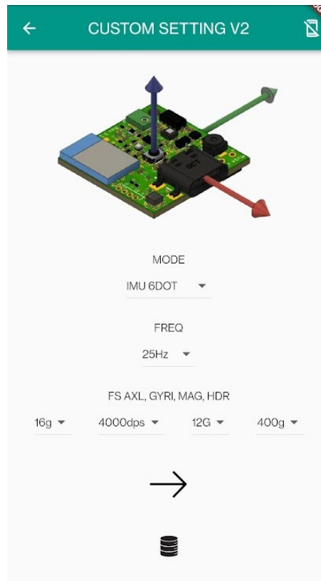
Figure 52 This screenshot of the V2SettingPage show that in this page the user can easily change modality, frequencies and full scale of the sensor.
