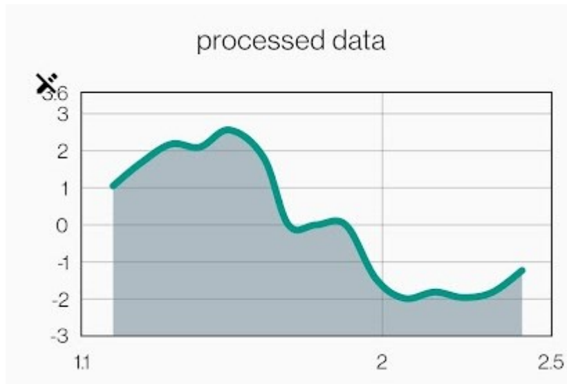
Figure 36 This image shows the final product of our pipeline, in which the raw signal from Figure 35 is processed and the portion of interest representing the execution of the Sit-to-Stand task is cropped.
