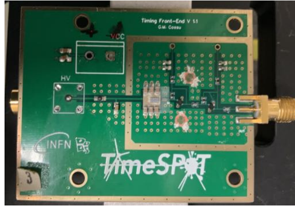
Figure 3.3: Electronic board for three Timespot sensors designed in Cagliari.
